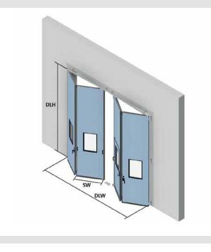
DLW = Daylight Width DLH = Daylight Height OH = Headroom SL = Side space Left SR = Side space Right D = Depth
