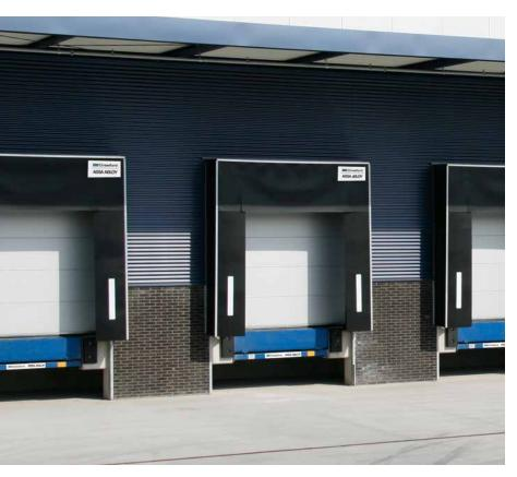
The Crawford 662 SMP is a curtain dock shelter which is available in a large variety of heights and widths. This model includes a self-adjusting top section which automatically adapts to different vehicle heights and vertical movements. The vehicle reverses into Crawford 662 SMP curtain shelter which seals it off with flexible side and top curtains, giving weather protection during the loading and unloading process.
